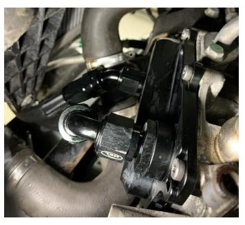
6. Install the bracket & shroud to the cooler. Fit the oil cooler to the car using the 3 factory bonnet latch mounting holes.
