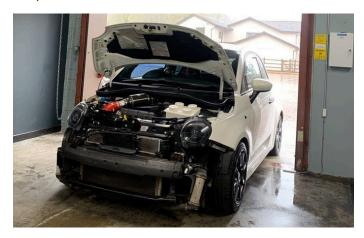
3. Locate factory heat exchanger and remove the heat shield.
