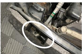
**8**. Connect the hoses to the engine take off plate, and feed through the space between the radiator/chassis rail and up through the new crash bar cut out.
