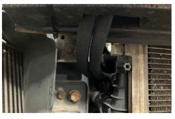
**9.** Pre-fill the cooler with OEM spec oil. Install the banjo adapters (being careful to support the cooler whilst doing so) to the top of the cooler.
