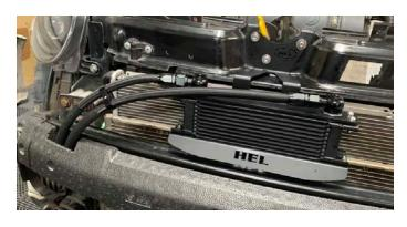
**9.** Start the car and check for leaks. Turn off the engine and check the oil level. Re-install the bumper & undertray. Lower the car off the jack stands.
