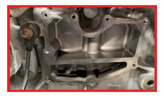
Install the HEL breather plate using a new gasket and the x8 supplied bolts. Torque using factory Ford specifications.
