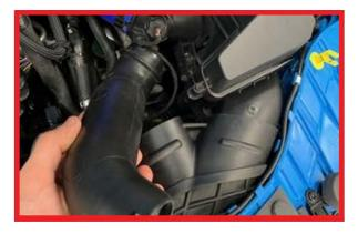
Remove the intake manifold and all required connections as per the OEM Ford instructions.
