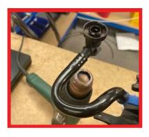
Lubricate and install the black manifold connector removed in STEP 7 to HOSE B. (We have found that these can sometimes be a very tight fit. If this is the case we recommend removing the sharp edges of the barb with sandpaper to ease installation and avoid damage to the hose.)
