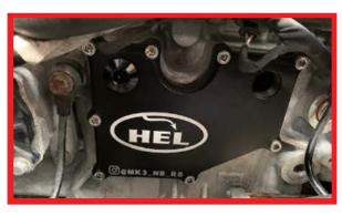
Using a heat gun carefully warm and remove the black manifold connector from the pipework attached to the factory breather plate.
